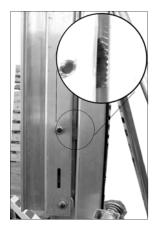
When the brake is engaged, it will be possible to see the Brake Cam acting on the adjacent mast section.
