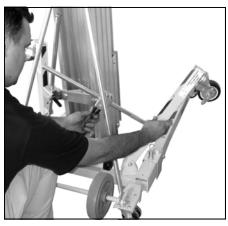
To replace the leg in the stowed position, pinch the locking mechanism release and fold the leg up.
