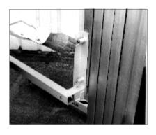
Disengage 2 spring-loaded pins. Rotate fork assembly 180 degrees. Engage 2 spring-loaded pins.
