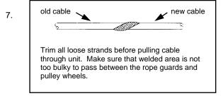
Bolt the new cable (looped end) to the top of the top mast
