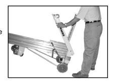
While holding the leg in the 90 degree position, slide the Leg Lock back towards the leg until the spring loaded plunger pin engages into position.
